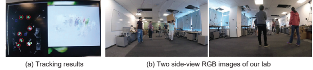
Figure 3. Sample tracking results of the proposed method. (a) Visualization of our tracking results. On the left of the screen is the top-down view with each numbered red circle representing one person. On the right is the real-time 3D point cloud. (b) We use two other RGB cameras to capture the corresponding side views of our lab.
